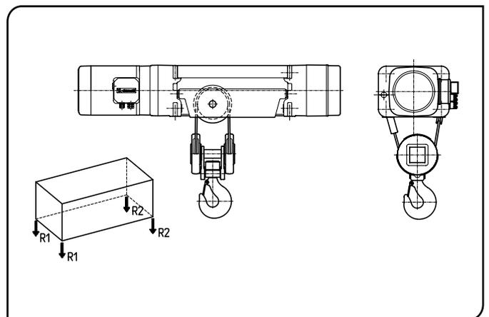
Single girder DST/N/S trolleys for DRH electric wire rope hoists – 2 rope falls version (2/1)
