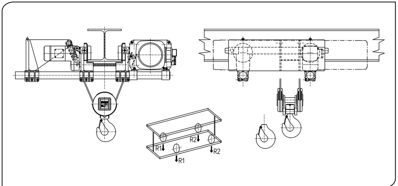
DRT double girder trolleys for electric DRH wire rope hoists set-down/suspended – 2 rope falls (2/1) and 4 rope falls versions (4/1)
