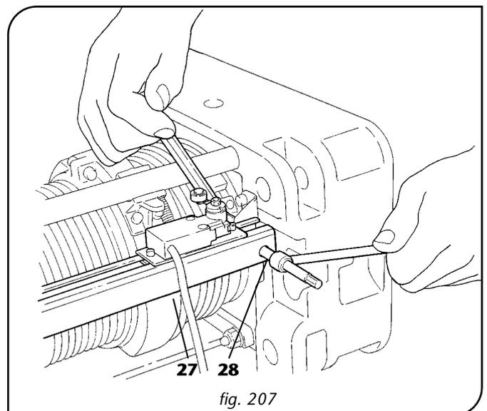
6.6.2 Lifting brake replacement (conical motor)
