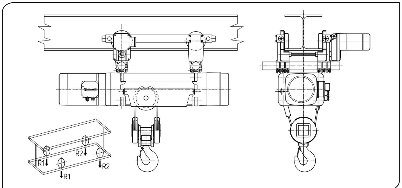
Single girder DST/R trolleys for DRH electric wire rope hoists – 2 rope falls version (2/1)
