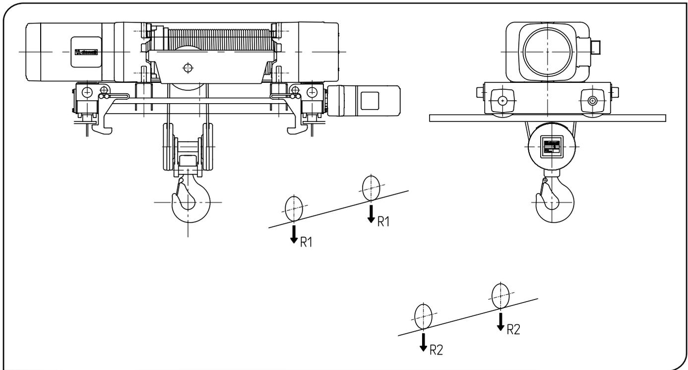
DRT double girder trolley for DRH wire rope hoist – Version with 6 rope falls (6/1) and 8 rope falls (8/1)
