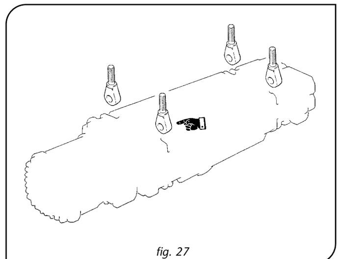
If the DRH electric wire rope hoist must be installed in set-down execution, the setting down of the hoist, in fixed position or on a trolley not supplied by DONATI, is foreseen with four eyebolts connected in the lower part of the carrying casing.
