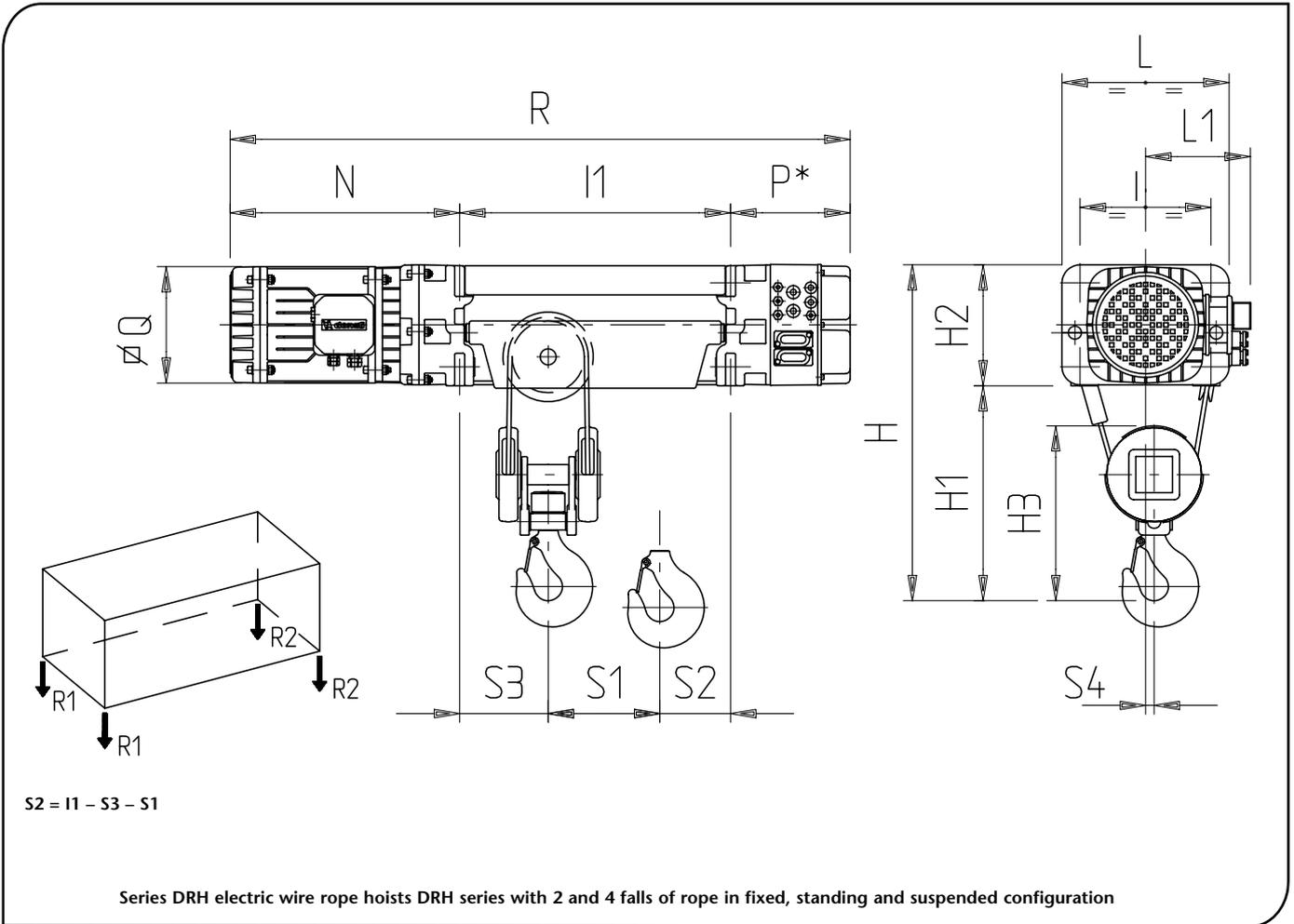
\* DRH3 and DRH4 with Low Voltage Control Box, the dimension P has to be: DRH3 = 330; DRH4 = 360
