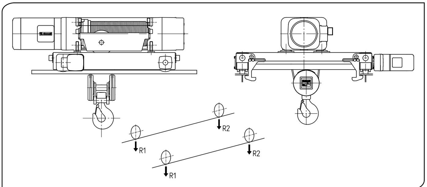
DRT double girder trolley for DRH wire rope hoist in trasversal position with 2 rope falls (2/1) and 4 rope falls (4/1)
