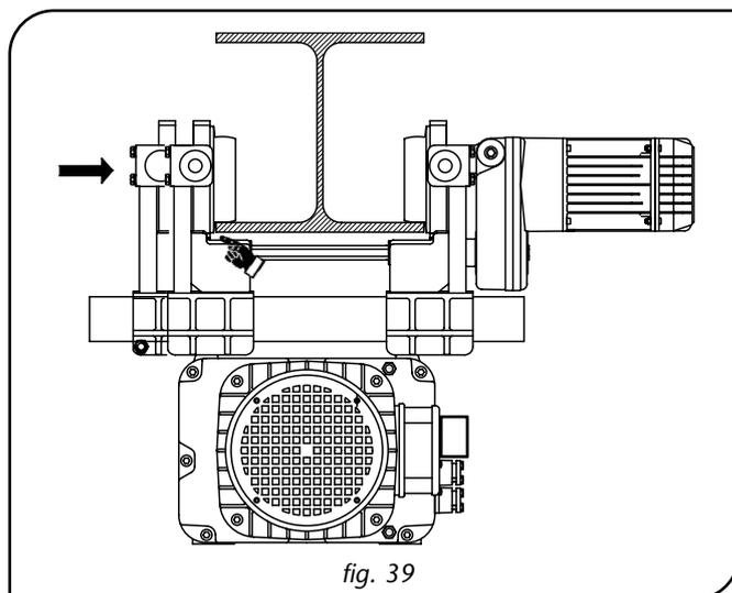
12. Check that all four sliding tracks of the trolley wheels are resting correctly on the girder and that between their edge and the wing of the section bar there is a clearance of 2 mm max. on either side (fig 40).
