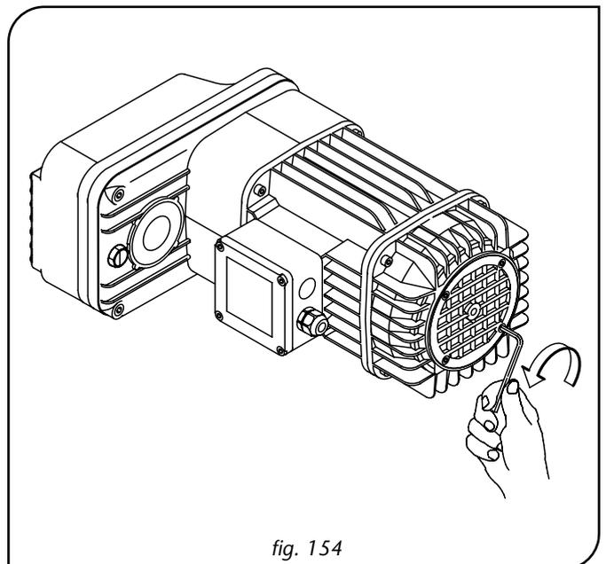
**A) - External adjustment of the braking torque:**
