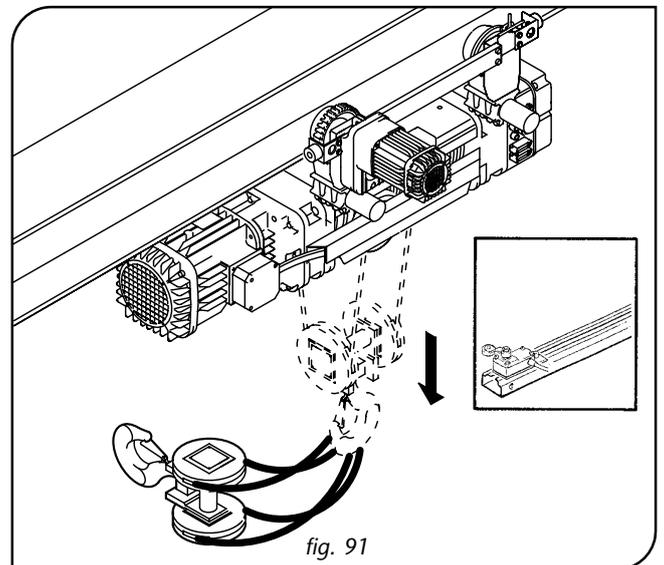
1. Check that the movements of the hoist correspond to the indications shown on the respective ascent and descent buttons of the push-button control panel:
