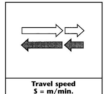
*It is the distance covered by the trolley in a minute of continuous running*
